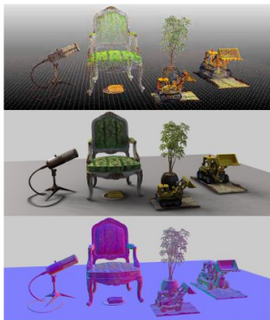
Figure 1. Multi-object composition and realistic relighting through our proposed relightable 3D Gaussian. From top to bottom: 1) optimized point cloud with BRDF attributes (colored with base color) 2) physically based relighting with shadow effects via point-based ray tracing, and 3) rendered normal map.
