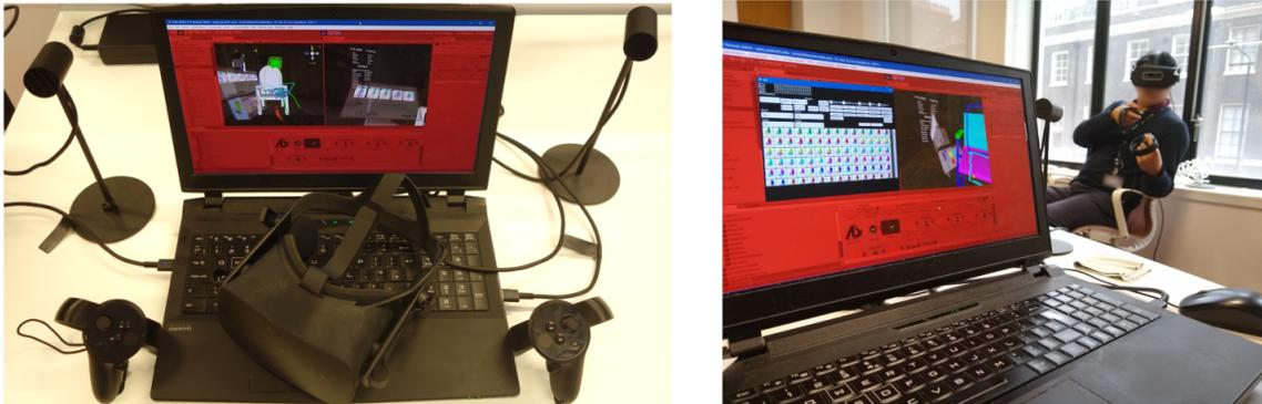
(a) Each participant used an Oculus Rift and Touch, performing all the experiments immersed in a synthetic scene. The experimenter uses the same laptop to perform the search by speech query.
