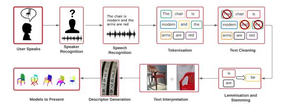
Fig. 3. The speech pipeline includes: speaker identification, speech recognition, tokenization, lemmatization, stemming, text interpretation, descriptor generation, selection of the proposed results.
