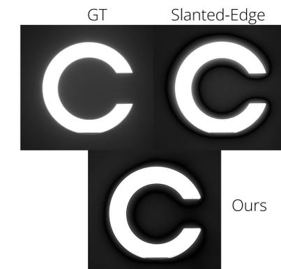
Figure 6. Top-Left: Captured image  $I(x, y)$  of C-shape with glare. Top-right: Image deglared by slanted-edge method. Bottom: Image deglared with our method.
