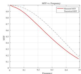
Figure 2. Example of a typical camera MTF vs frequency curve.
