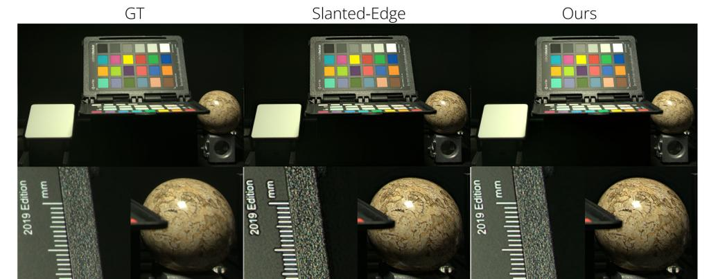
Figure 5. Left: Original image. Center: Image deglared with slanted-edge MTF measurement. Right: Image deglared with optimisation-based MTF measurement.
