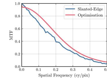
Figure 4. MTF vs spatial frequency for slanted edge and optimisation estimation methods.
