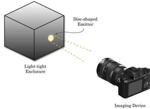
Figure 3. Diagram of the capture setup for low-frequency MTF estimation
