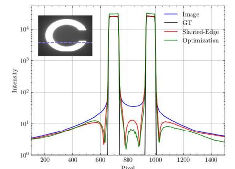
Figure 7. Intensity of pixels (log-scale) across a horizontal scanline in the images from Figure 4, showing the original and deglared images obtained by Slanted-edge and optimization (ours) methods.
